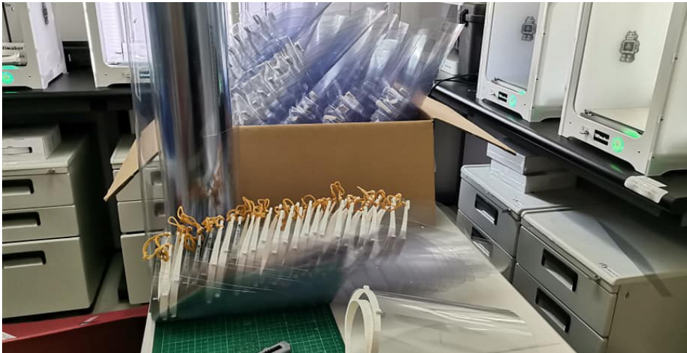
LIKHA FabLab's 3D printers, vacuum forming machines produce the Red Spartan Face Shields using PLA Filaments and PVC Sheets.
